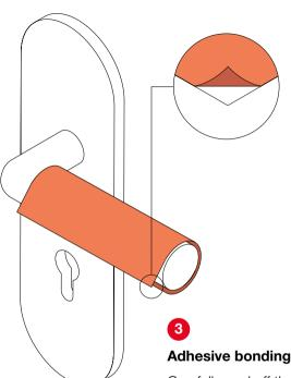
Carefully peel off the backing paper by pulling it flat back on itself and stick the tape on so that the beginning and end of the tape meet at the bottom of the handle. Slide the tape from the middle outwards into final position.
