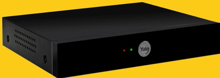
A Hybrid DVR is a Recording device that can accept more than one type of video signal input. The most common video signals used today are analogue BNC & IP Network Cameras. The advantage of having a Hybrid DVR is the ability to use analogue cameras, while adding IP megapixel cameras to areas that need more detailed monitoring through better image quality.
